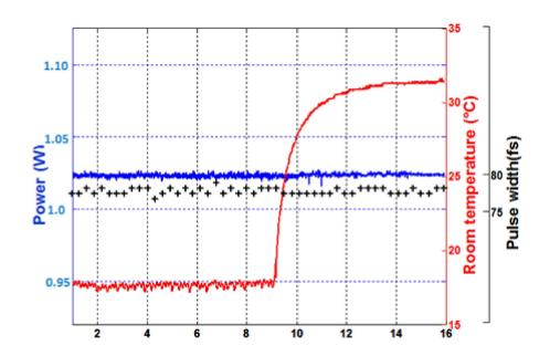
**OptaPower™** is designed for those customers that are trying to measure incredibly small signal levels and require hours of data acquisition. It ensures ultra-stable power and pulse width performance from the Carmel for hours irrespective of any variation in the ambient temperature. Over a room temperature change of 17 to 32°C, OptaPower provides a factor-of-two improvement in the rms pulse width stability and an order of magnitude improvement in rms power stability.
