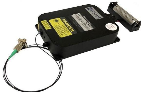
In addition, the latest desktop version of the Mendocino platform will be on display, targeted for the optical communications test and measurement sector. With an output at **1310 nm**, pulse widths of **< 0.3 ps**, and **triggering jitter as low as 200 fs**, this source is perfect for new generation data center transceiver component testing and photodiode characterization.
