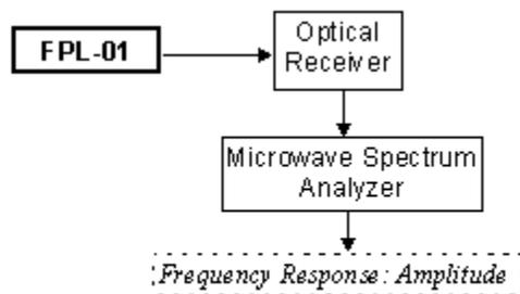
**Figure 6 – Measuring Frequency Response of an Optical Receiver**
