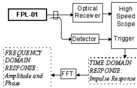
**Figure 5 - Measuring High Speed Receiver Performance**
